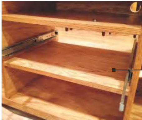
STEP 23. You can then attach the drawer rails
